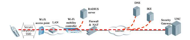
The diagram above shows the functional entities required for secure UMA service over a corporate WLAN.
